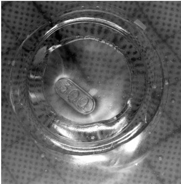
Figure 2. Closer view of the posterior patch region of a shell exposed to Betadine pocket irrigation and removed after 16 months. The photograph reveals no signs of patch delamination or disruption at the patch-shell interface.
